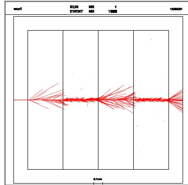
Cut in range: sampling: LAr(4mm) Pb(4mm). Protons 500 MeV. Geant4
