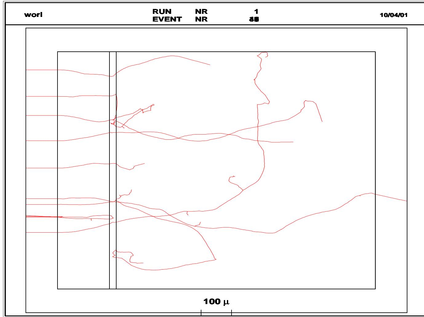
Distribution of energy deposit by 1 MeV electrons in Al-Au-Al slab :
