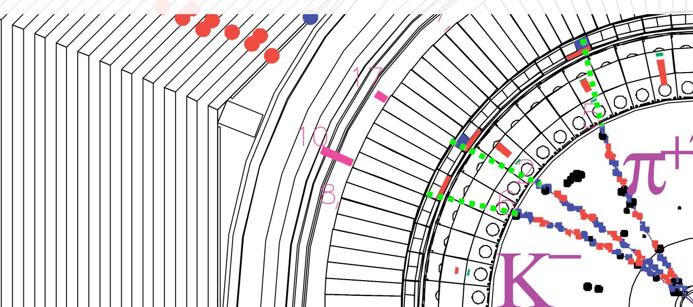
Muon identification using geant4e: Swim track from outer edge of drift chamber through muon detector (with Kalman fitting to matching hits, if any)
