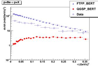
Fig. 9. Differential cross section, as a function of the transferred fourmomentum, for the target diffraction process. Protons of p = 450 GeV/c impinging on a beryllium target collected by the HELIOS experiment are compared to GEANT4 version 9.5. $\beta$  simulation. Results obtained with the qurk-gluon-string (QGSP\_BERT) and Fritiof (FTFP\_BERT) models are shown.
