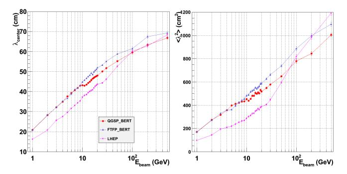
Fig. 5. Simulation of pion induced showers in an iron-scintillator calorimeter obtained with GEANT4 version 9.5. $\beta$ . The shower depth (left) and shower length (right) of three different physics lists (LHEP, FTFP\_BERT, QGSP\_BERT) are compared.
