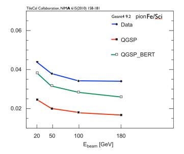
Fig. 3. Lateral leakage for the Tile calorimeter. The ratio between the energy released in the module displaced with respect to the beam axis and the central module is shown as a function of beam energy. The modules are about 30 cm wide. Test-beam data are in blue, QGSP\_BERT is shown in green and a physics list without a cascade model is shown in red.
