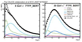
Fig. 7. Longitudinal profile obtained by the CALICE collaboration with the test-beam data of a tungsten, silicon digital calorimeter. Pions beam with two energies are shown: 8 GeV (left) and 30 GeV (right). The simulation is obtained with GEANT4 version 9.3 and the FTFP\_BERT physics list. For the simulation the contribution to the shower profile of each particle species in the profile is also shown. Courtesy of the CALICE collaboration [5].
